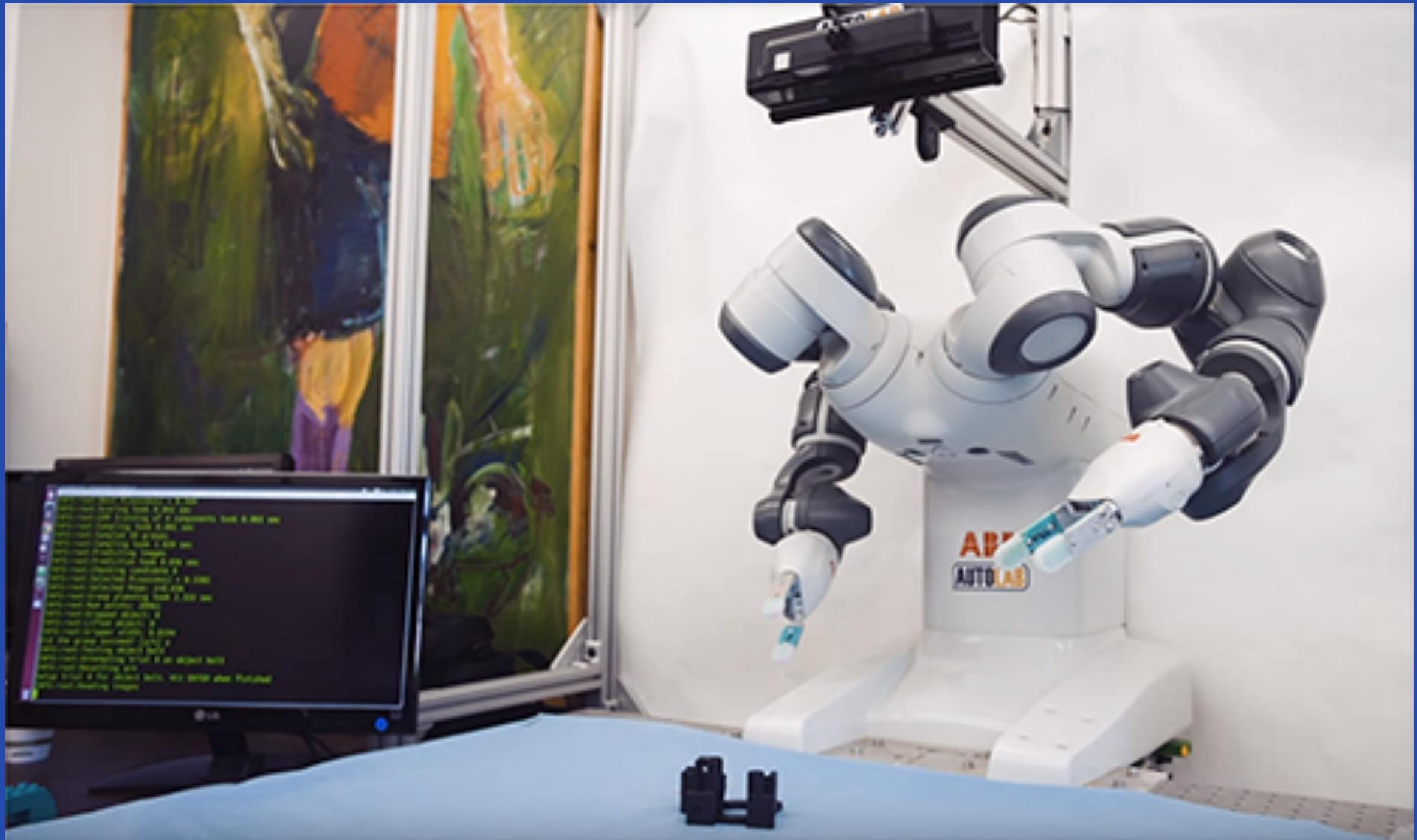
A robot manipulates objects it has never encountered before after researchers teach a neural network how to recognize objects from millions of 3D models and images. (Photo courtesy of University of California, Berkeley)
